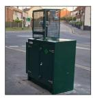
TMBC has installed an Air Quality Monitor at the Western Road/Sevenoaks Road roundabout. It will be there for at least a year to collect data on the quality of air that we are breathing in - the level of Particulate Matter (PM 10) that can end up in our lungs.
