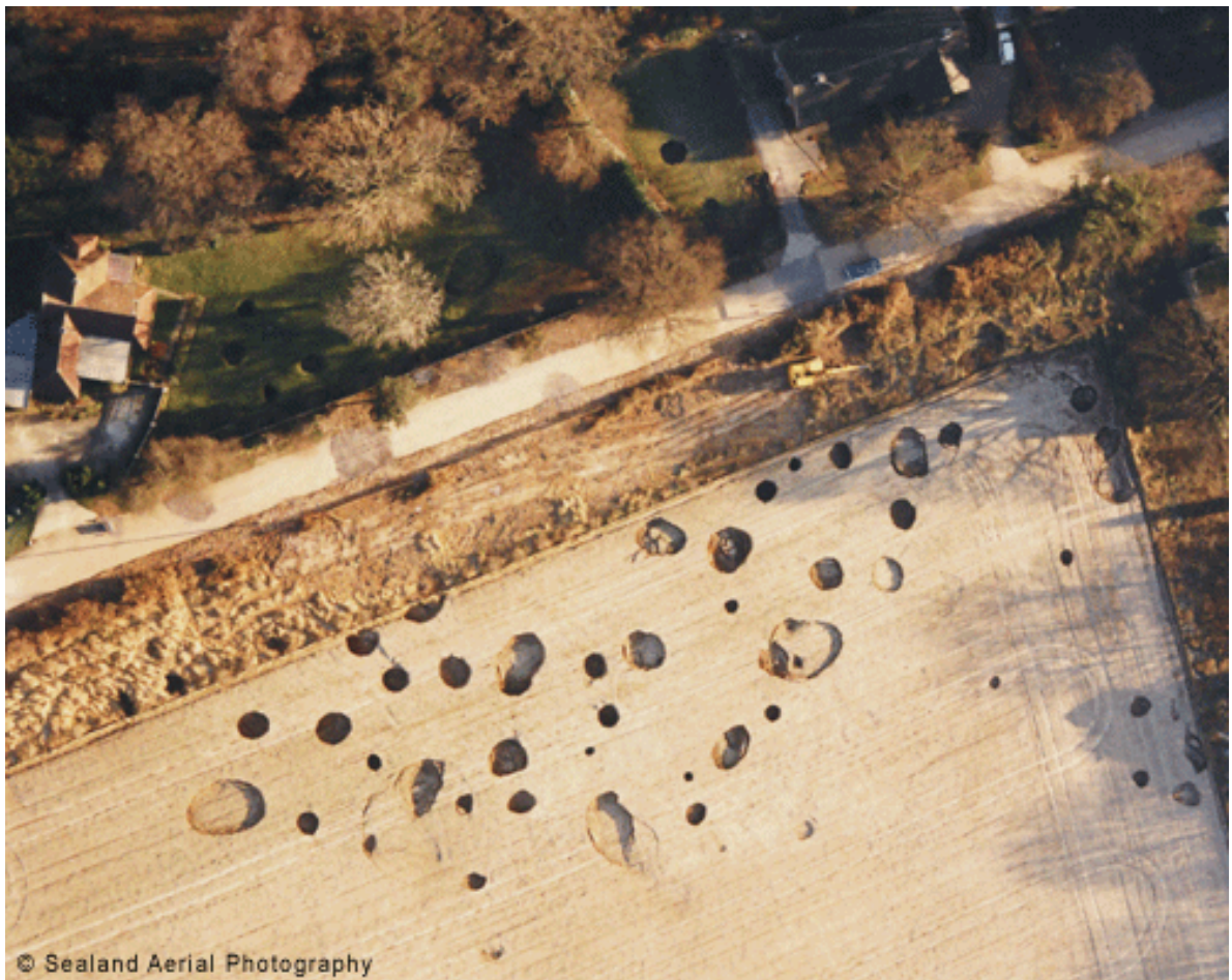
Sinkholes formed on Chalk due to a burst water pipe at Fontwell, Sussex. © Sealand aerial photography.
